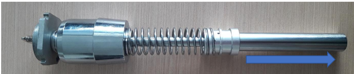
Figure 9: System and Strike Direction to Remove Impact Plunger
