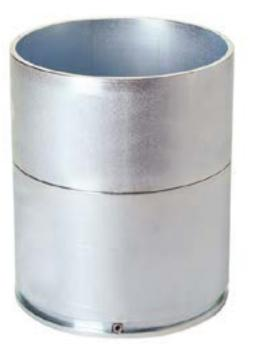
The 6" or 150mm compaction mold assembly is used for preparing test specimens with compactors. The mold is designed to be used with rotating or stationary mold models. A mold is machined from seamless tubing and plated. Comprised of a base plate, mold cylinder and extension collar.
